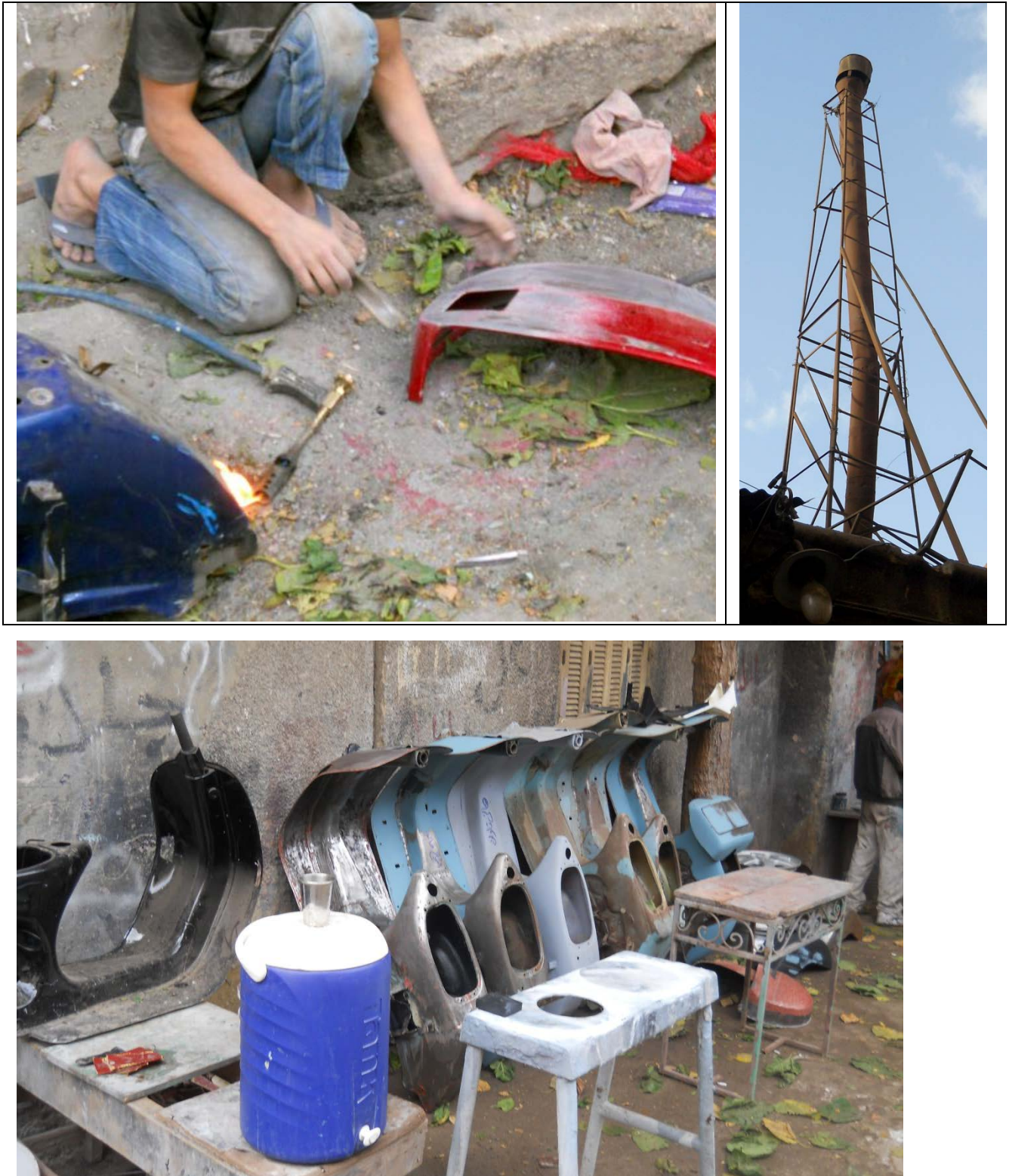
Fig 2-10 maintenance or even production of motorcycles in souk el silah replaced original Arms casting, an activity which is inconsistent with the historical nature of the area degrading its visual quality. welding may cause fires due to unsafe process, specially by children or uneducated young assistants, welding means existence of flames and combustible fuel in addition to Oxygen cylinders,
