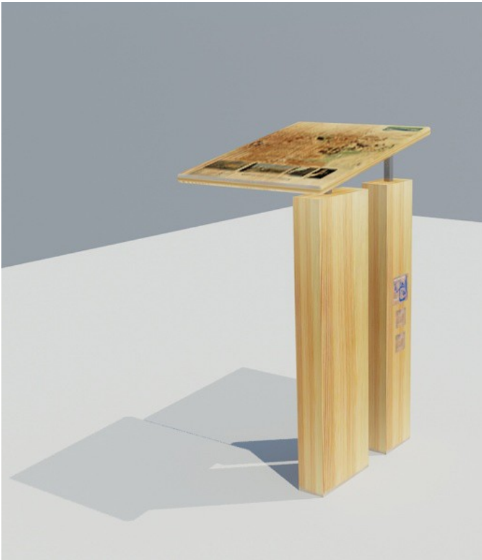
Fig. 102: The Action Area sign 3D presentation, Double poles in pine wood and the Action Area map printed on wood
